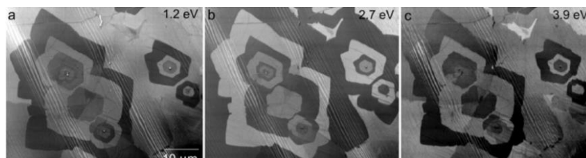
Figure 1: Graphene multilayers observed by ultra-low energy SEM: 1.2 eV (a), 2.7 eV (b), 3.9 eV (c)
